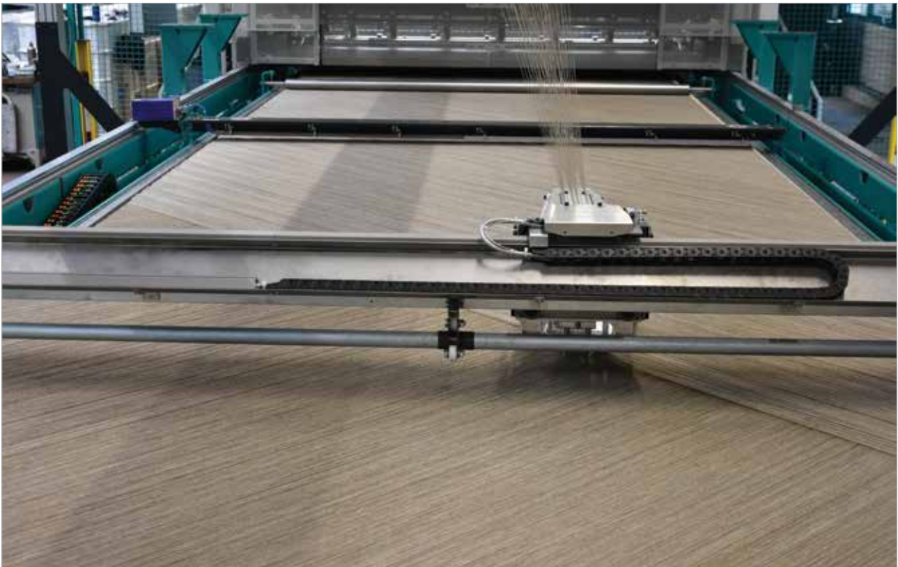
Flax yarns being laid at angles on Karl Mayer's Cop Max 4.
