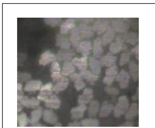
Figure 3: Cross-section of bamboo viscose rayon
