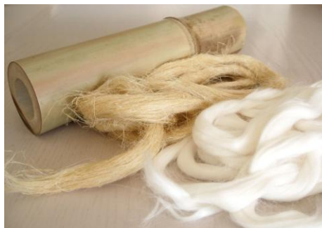
Figure 1: Fiber extracted from bamboo by mechanical method.
