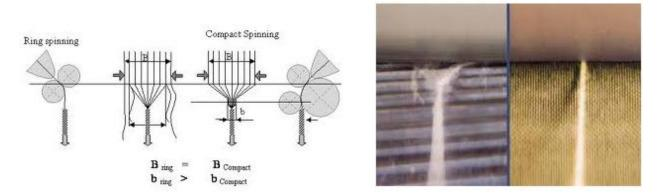
Also the spinning triangle is the major weak place in yarn formation zone and therefore most of the end breaks in ring frame are occurring in spinning triangle and which is largely influencing the machine efficiency. Therefore it needs to have control over formation of spinning triangle and which is made possible by compact spinning.
