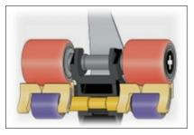
According to Stahlecker, RoCoS 1 is suitable for 100 % cotton, cotton blends and 100% synthetic fibers with maximum staple length of 60 mm. RoCoS 2 is suitable for 100% wool,100 synthetic and wool/synthetic blends having minimum staple length of 50 mm. As RoCoS does not requiring air suction, air piping, perforated drums or apron and therefore there is no extra power and maintenance is necessary.
