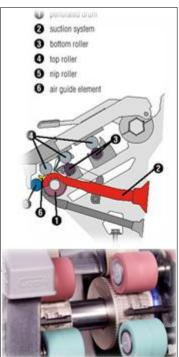
drafting system. The suction under the tube creates the air currents through slot and lattice apron which are responsible for condensing and perfect parallelization of fiber strand. The suction air pressure, size of slot, speed of apron, number of holds in the lattice apron has an influence on condensing action.
