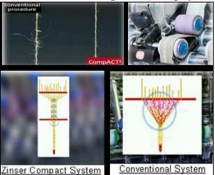
quality. Therefore for cotton compact spinning process, 0-4% overfeeding is required as per raw material.
