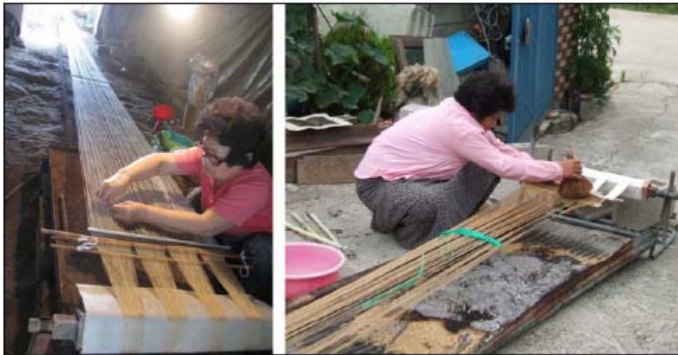
Figure 9: (Left) Starching ramie yarns over a gas-heated metal plate, Hansan. (Right) Starching hemp yarns over burned rice husks, Andong. Images by author.
