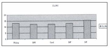
It observed from the table 1 to 7, in most of the mills 50% span length deteriorate in blow room and carding. But as compare to 2.5% span length this deteriorations very less
