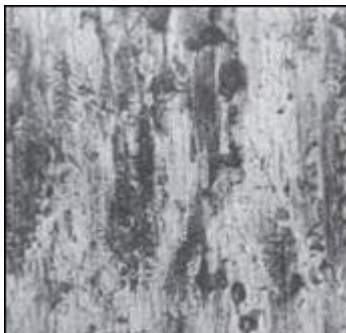
Smearing on the surface of a roller from a spherical roller bearing
