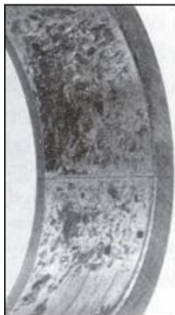
Spherical roller bearing inner ring with fretting corrosion and a transverse crack right through the ring. The fretting corrosion has caused the cracking
