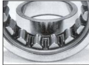
A cylindrical roller with smear streaks in the inner ring raceway and on the roller
