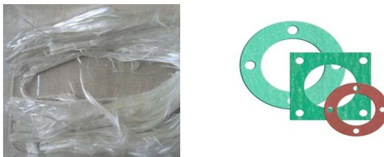
Fig.6. (From left) Asbestos fibres, CAF ( Compressed Asbestos Fibre) Gaskets
