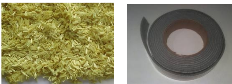
Fig.8. (From left) Aramid fibre segments, Aramid fibre gasket tape
