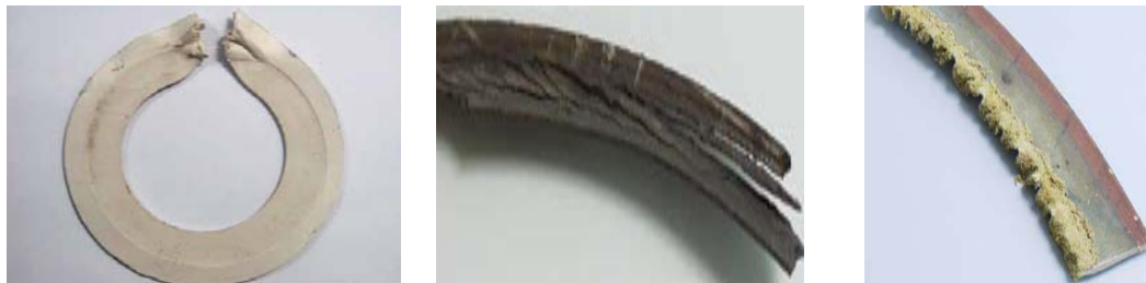
Fig.14. Various gasket defects
