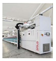
• FLEXIROTORS 3000 automatic rotor spinning frame, specifically designed to meet the
