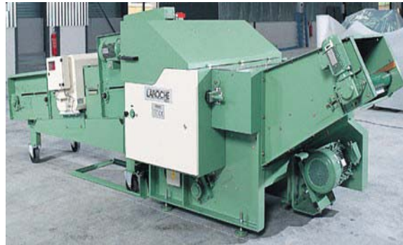
STARCUT: High production rotary cutter for all textile wastes.
