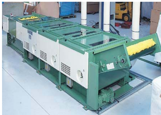
CADETTE: Machine designed to open all types of textiles wastes such as threads, woven, knitted and non-woven materials.
