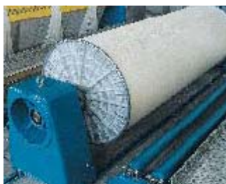
Fig: 14 Unwinding devices for section warping beams.
