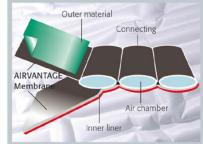
Airvantage membrane system, specially developed for the construction of permanently airtight and breathable chambers, is based on the same PTFE technology as Gore Tex.
