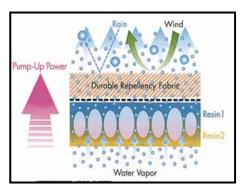
**Entrant G II:** Toray has developed a high performance waterproof breathable fabric Entrant G II. It is a microporous coating of polyurethane developed with importance given to high water pressure resistance and high moisture permeability.
