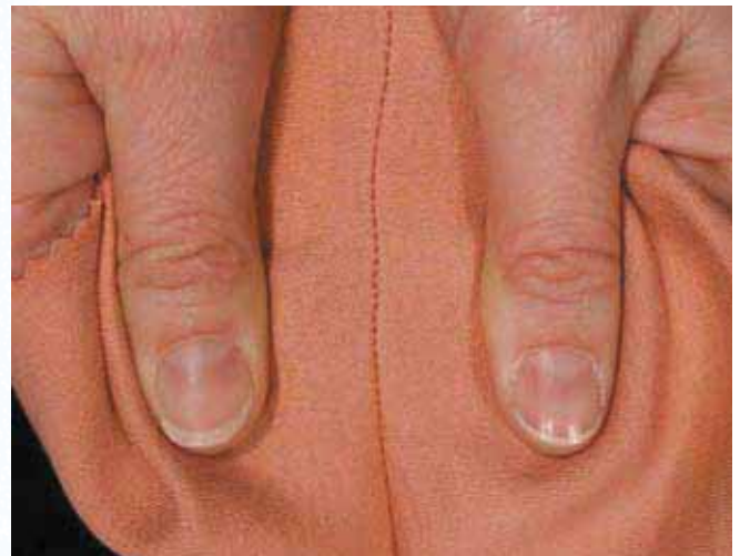
Seam sample manual stress test
