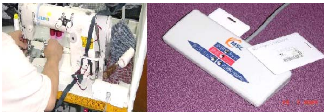
There will be a low-cost tag smart card and reader next to each of the sewing machines for recording the details of work by each staff.
