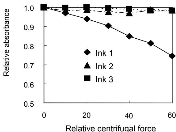
Fig. 1 Sedimentation properties of three inks
