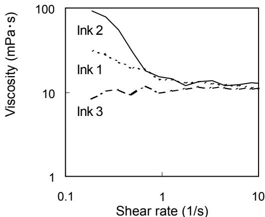
Fig. 4 Viscoelasticity of three inks
