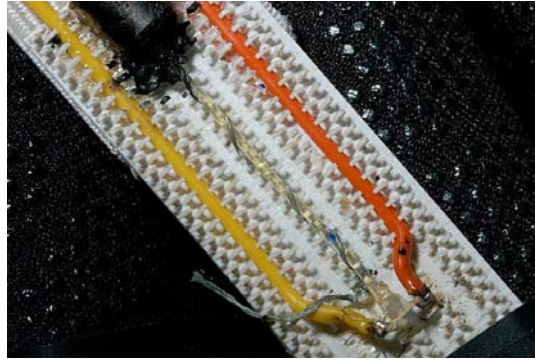
Fig. 5: Auxetic Optical Sensor mounted on a Velcro strip
