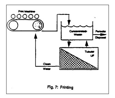
The best membrane for this application is the one inch FEG tube used in a modified batch mode. It readily handles the high viscosity at the end of the run. It can be mechanically cleaned with a sponge ball or pig and it has a long membrane life.
