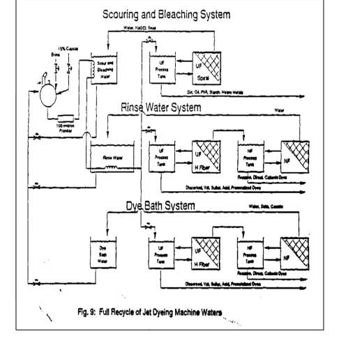
The kidney setup continually removes oils, greases and dirt, concentrating them in the membrane systems process tank, and recycles the surfactant laden permeate back to the scouring bath. The best process mode for batch scouring operations is modified batch (Figure 9.)
