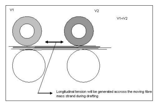
Measurement of drafting force is a useful aid raw material selection, optimization of spray oils used in cotton, optimization of crimp and spin finish level in synthetic fibres. The frictional force acting on fibre assembly during drafting can be determined experimentally by measuring the total resistance of fibre assembly. The frictional force depends on relative fibre velocities and density distribution.
