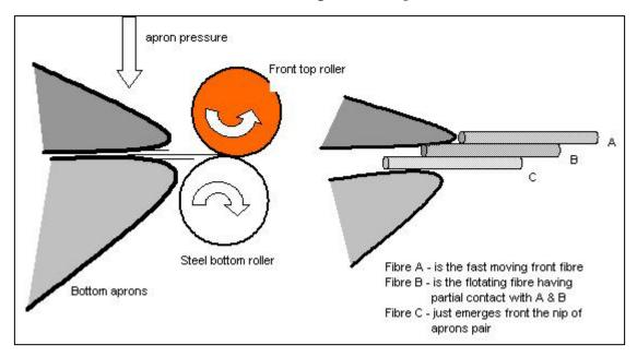
Under normal conditions the fast moving fibre A should over come the resistance offered by fibre B which is a floating fibre at the same time fibre B should overcome the frictional resistance offered by fibre C which in turn gripped by the apron pairs .
