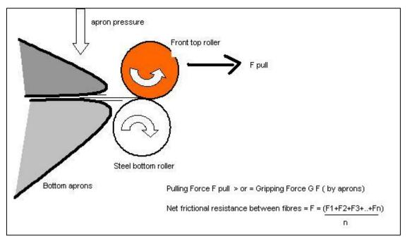
Net frictional resistance between fibres =  $F_F$ Net frictional resistance offered by aprons over fibres =  $F_A$
