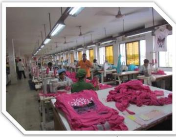
Our sewing section consists of 12 complete sewing lines in two separate floors. Each line is equipped with 20 to 25 sewing machines
