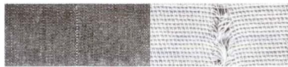
Running defect/ Repair warp thread
